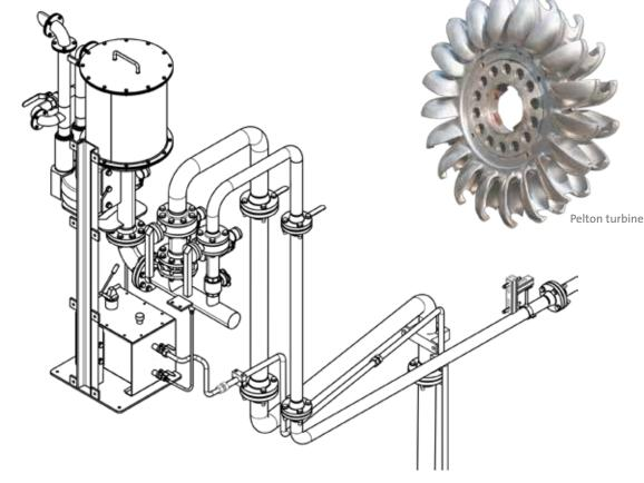
Example drawing of an Oil Mist Separator for a hydro turbine
